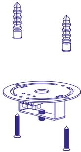
**2** Thread the power cord through all the parts as shown and connect Power to terminal block.
