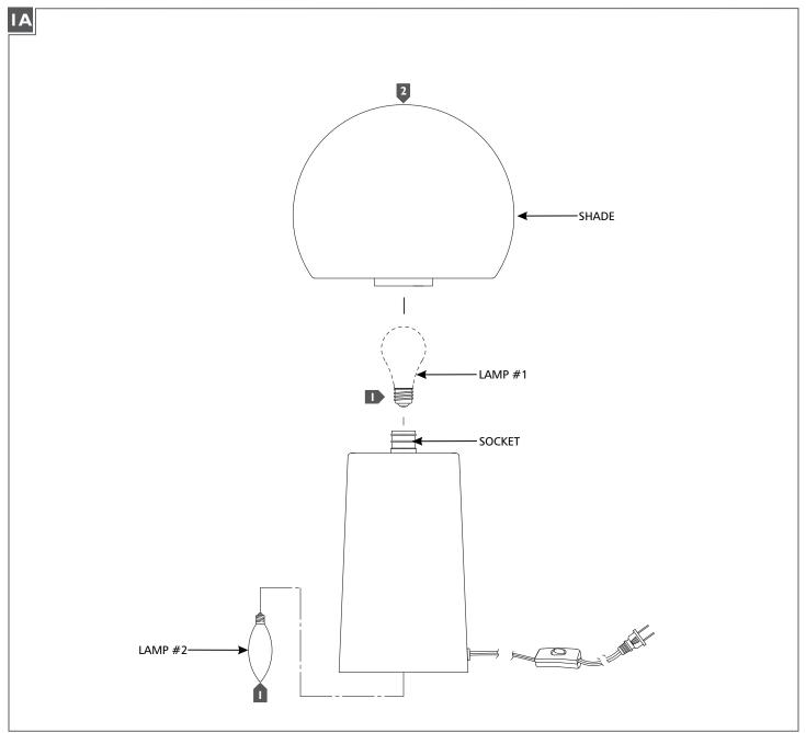
Screw the lamps into the sockets. Refer to the labels on the lamp sockets for Max Wattage Information.
