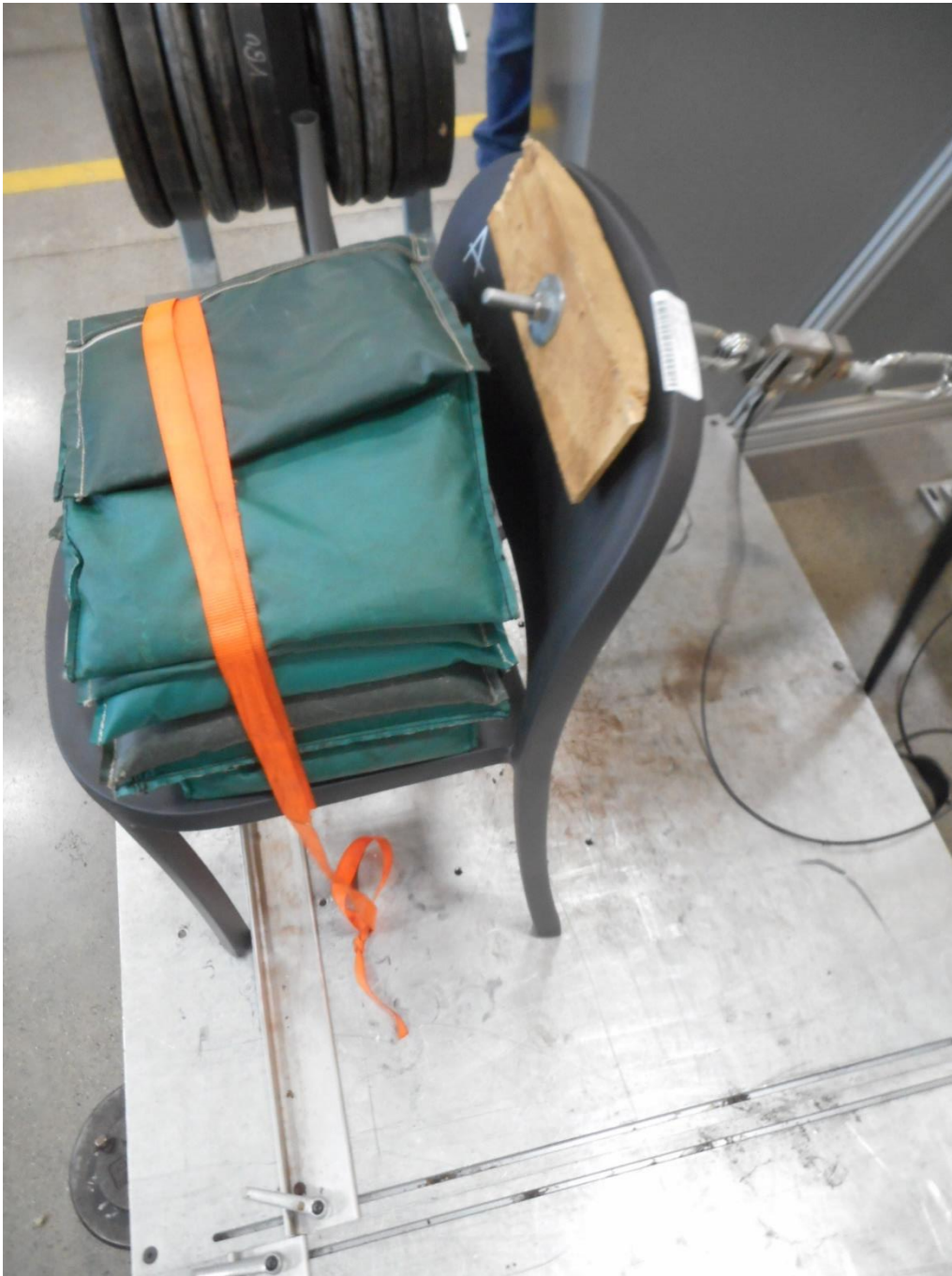
Backrest Durability Test – Cyclic
