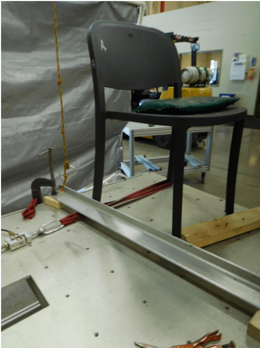
Leg Strength Test – Side Load
