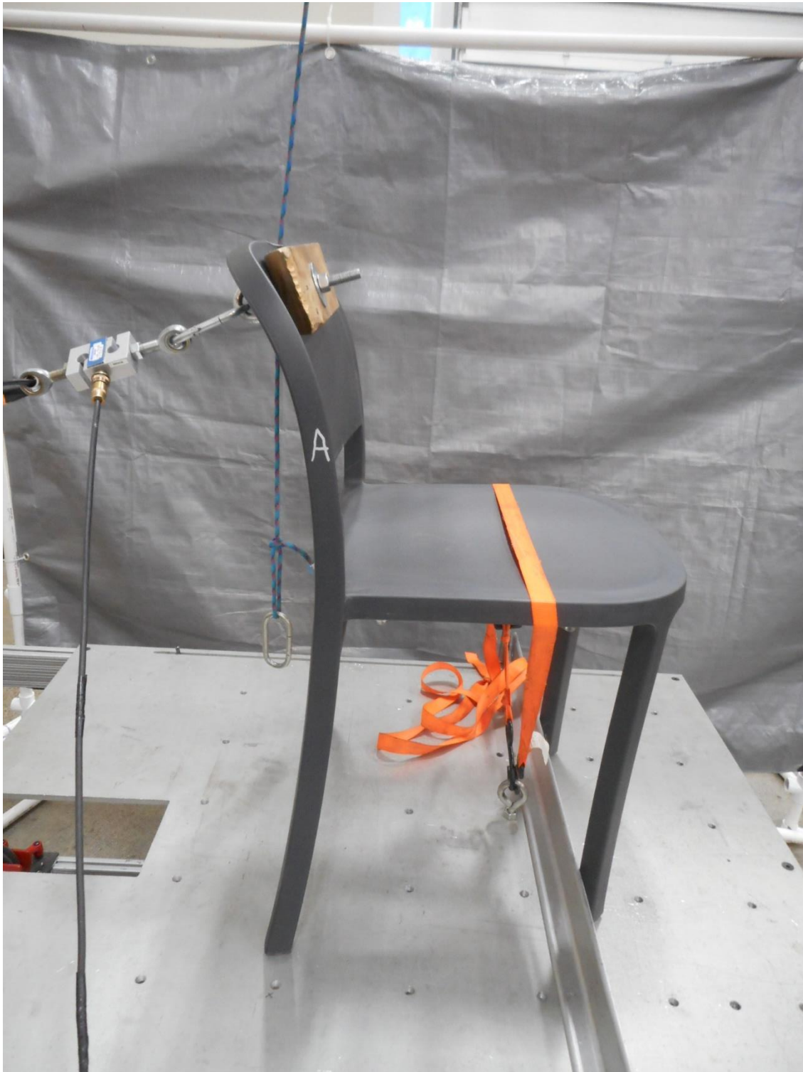
Backrest Strength Test – Static
