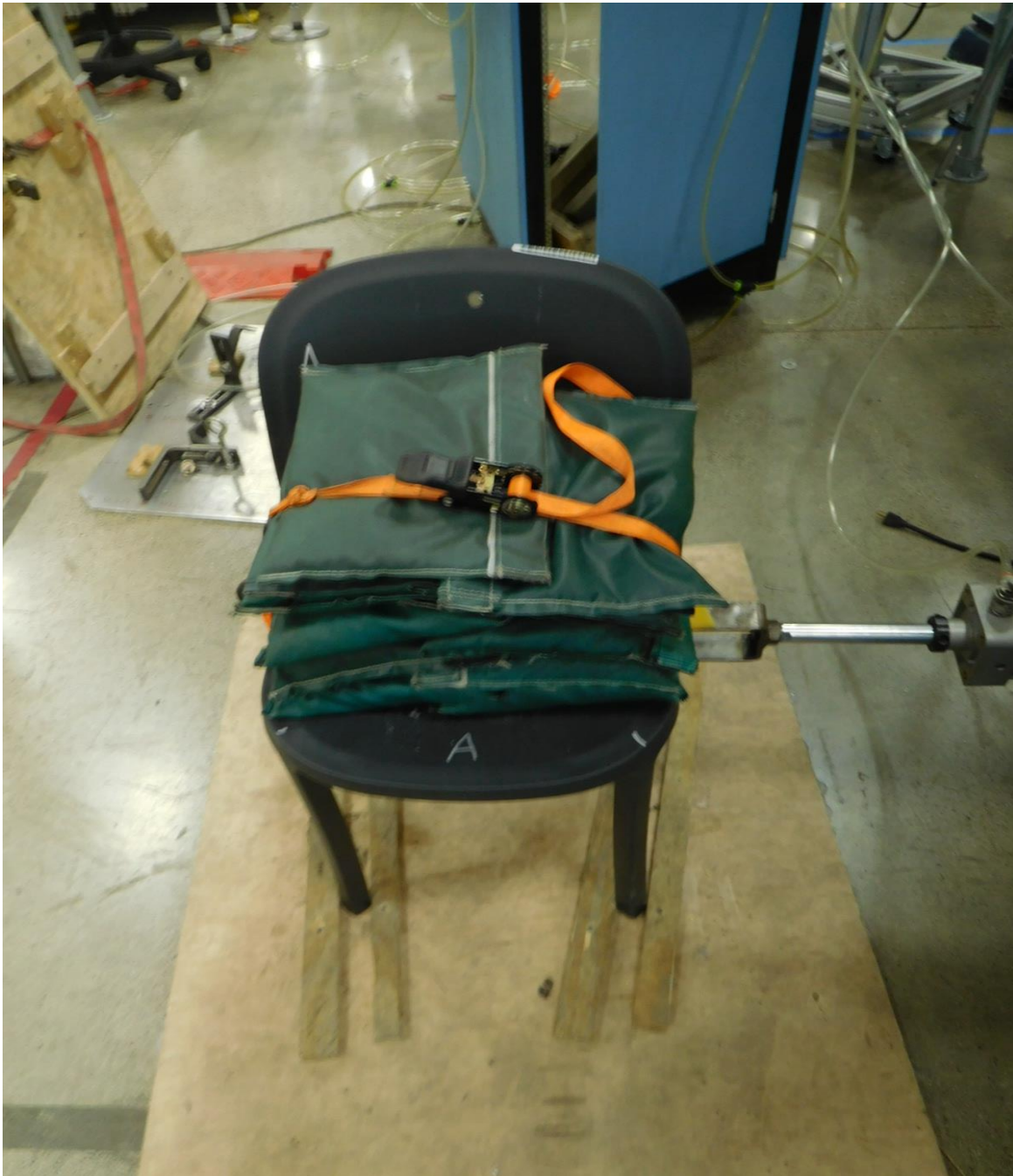
Structural Durability Test – Cyclic
