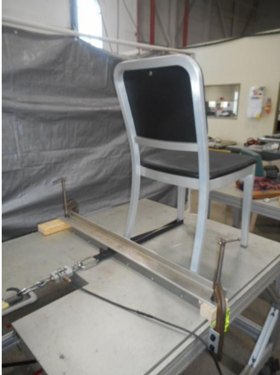
Leg Strength Test – Front Load
