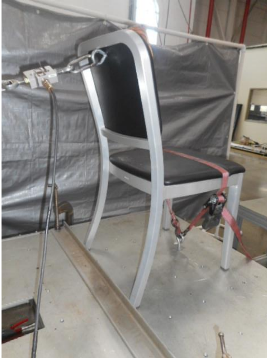
Backrest Strength Test – Static
