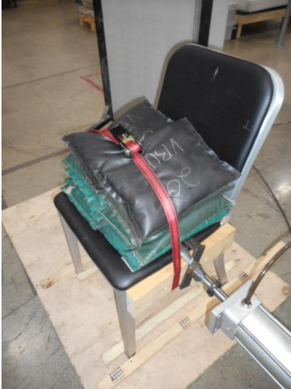
Structural Durability Test – Cyclic
