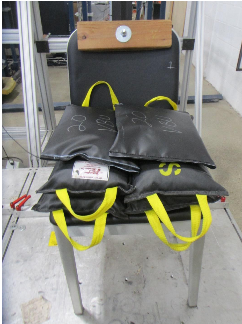
Backrest Durability Test – Cyclic
