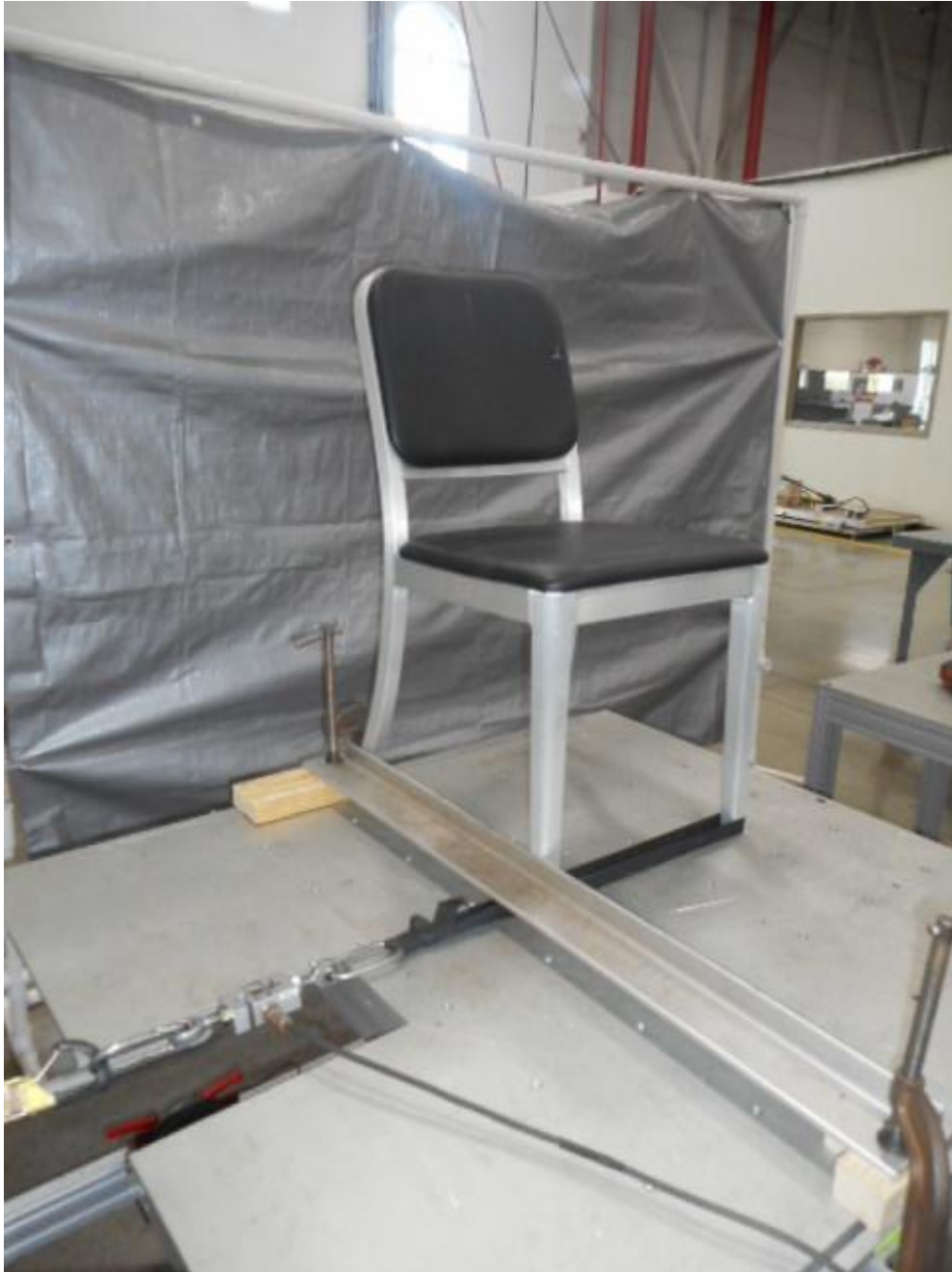
Leg Strength Test – Side Load
