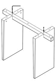
Insert hexacon screws and tighten using the allen key.
