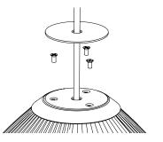
Assemble the top part by placing the hat (4a) on top of the shade and attach with the screw (4b). Make sure it's properly tightened.
