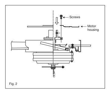
Re-install top of the motor housing back to the motor assembly. (Fig. 2)
