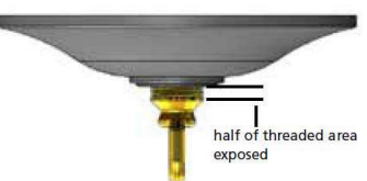
Drawing 2 – Canopy Adjustment
