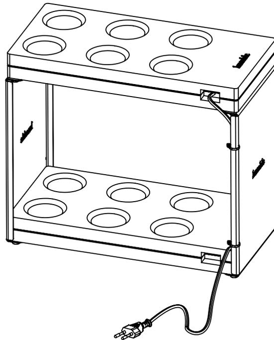
Guide the cable(s) using the tie-wraps.
