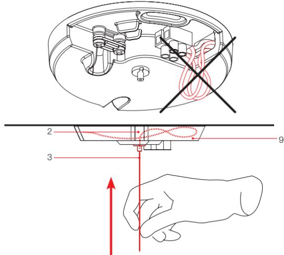
If you feel you have pushed the metal cord too high, you can recover it by pressing the cord clip shown in the figure. to release the stop. During this step, hold the body of the lamp to prevent accidental dropping.
