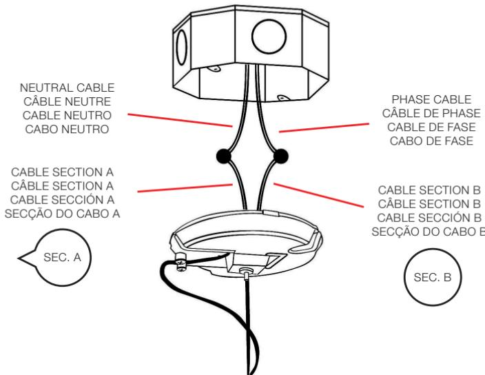
Feed the power cables from the ceiling into the clamp (8), guiding them through the slot. Then attach the base to the ceiling using the grips supplied with the kit.
