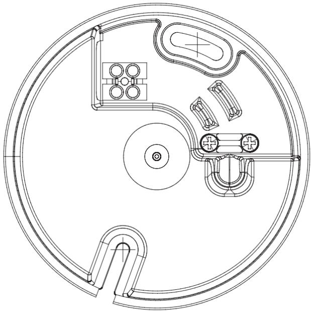
Make electrical connections by connecting the neutral cable with wire having section A and the phase cable with the one having section B.
