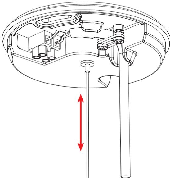
Loosen the screws on the wire clamp (7) to allow the passage of the power cable. Insert the wires into the terminal (8) and tighten. Tighten the wire clamp against the external sheath of the wire. Press the ceiling rose (2) gently against the base (1) until it clicks into place.
