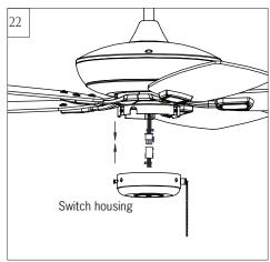
Connect the plug from fan with the plug from switch housing. Be sure plugs connection clasp together completely.
