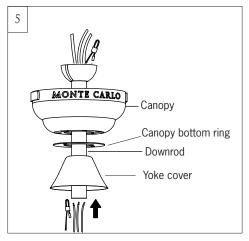
Place downrod over canopy, canopy bottom ring and yoke cover. Thread lead wires and safety cable from motor assembly through downrod.
