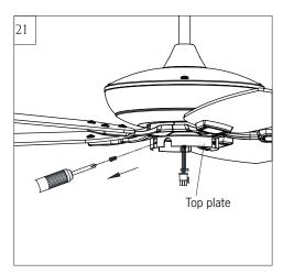
Remove the 3 set screws on top plate of switch housing, keep screws.
