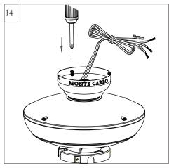
Reinstall the 3 set screws remove in step 11. Tighten screws securely.
