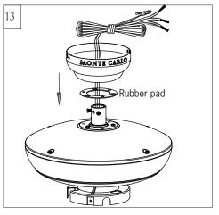
Place canopy and rubber pad over lead wire and safety cable and align the larger holes in canopy and holes on rubber pad with the set screws on yoke.
