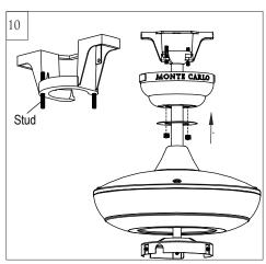
Lift Canopy allowing the 2 studs to protrude through the canopy.
