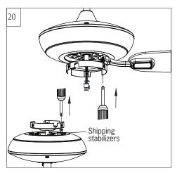
Remove shipping stabilizers from motor assembly.
