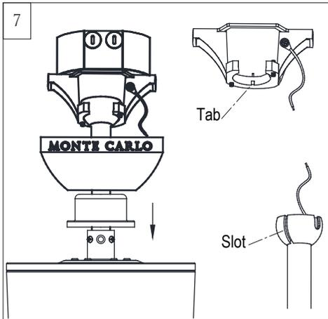
Install ball end of downrod into mounting bracket opening. Align (engage) slot on ball with tab on mounting bracket.
