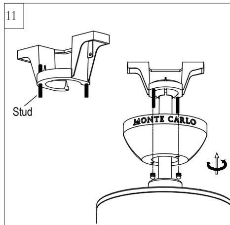
Lift Canopy, allowing the 2 studs to protrude through the canopy. Install knurled nuts provided and tighten the knurled nuts securely. The canopy should adjust for any irregularity in the ceiling or outlet box. Make sure the studs protruding from the bottom of the Mounting bracket are installed with threads all the way through the bracket.
