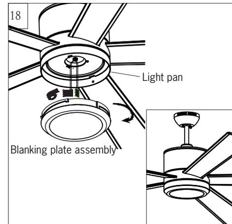
Isolate the quick connects with electrical tape. Attach blanking plate assembly onto light pan by locating dimples in light pan with grooves in blanking plate and twist clockwise until tight.
