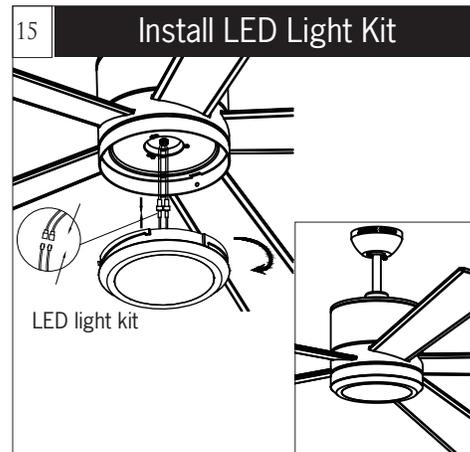
Connect white wire from fan to white wire from LED light kit and then connect blue (or black) wire from fan to black (or blue) wire from LED light kit. Attach LED light kit to light pan by locating dimples in light pan with grooves on the LED light kit and twist clockwise until tight.
