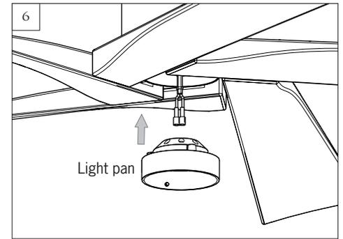
Place light lead wires over the light pan.
