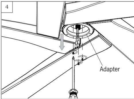
Remove 3 set screws and remove the adapter. Keep screws.
