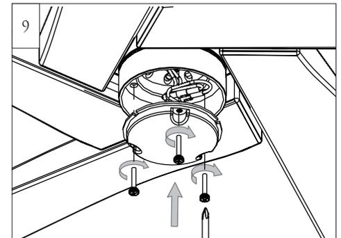
Install the light fixture onto light pan using set screws provide.
