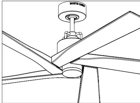
Install a lexan shade. Attach a lexan shade by locating dimples in light pan with grooves on the shade and twist clockwise until tight.
