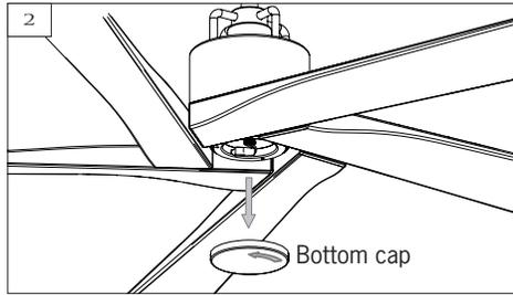
Remove the bottom cap by turning counterclockwise.
