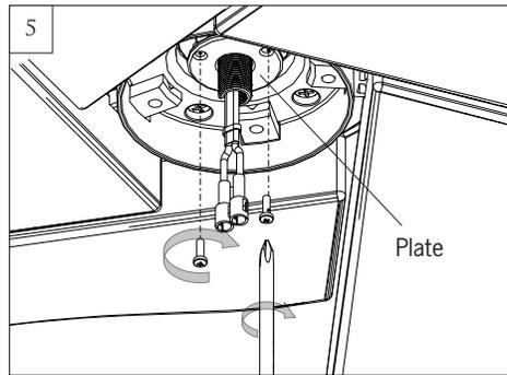
Partially install 2 set screws on the plate with motor using the screws which are removed on the installation step 4.
