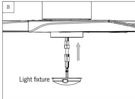
Install light fixture. Lift light fixture up, Connect white wire from fan to white wire from LED light fixture and then connect blue (or black) wire from fan to black (or blue) wire from LED light fixture.
