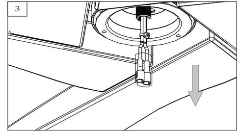
Remove the insulated shrunken sleeve from light lead wires using a suitable tool.
