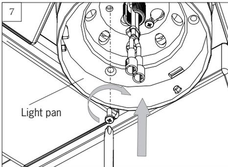
Install the light pan. Align the key hole slots on light pan with the 2 set screws and turn it clockwise until tight. Install the other screw which is removed on the installation step 4. Tighten all set screws securely.
