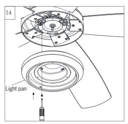
Attach light pan onto the plate on motor, Place light pan over the lead wires from fan, aligning the keyhole slots on the light plate with the preassembled screws on the plate. Twist clockwise till lock. Reinstall the screw removed in step 13. Tighten all screws securely.
