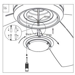
Connect white wire from fan to white wire from LED light kit and then connect blue (or black) wire from fan to black (or blue) wire from LED light fixture.
