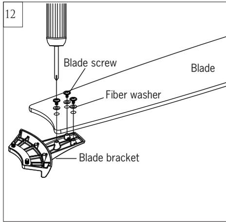
Install blade bracket with blade by using blade set screws and fiber washers provided. Tighten screws securely. Repeat this process for remaining blades.
