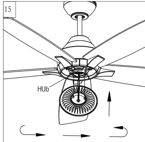
Install the LED light fixture onto the hub on the fan. Place light lead wires in the hub and attach LED light fixture onto the hub by locating ridges in the LED light fixture with the grooves on the hub and twist clockwise until tight
