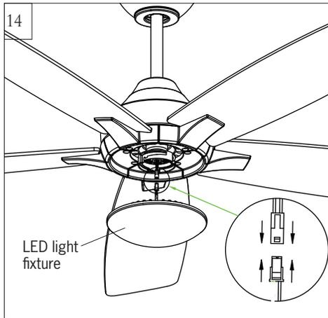
Connect the light lead wires from fan to LED light fixture with a quick connector as shown in the illustration.
