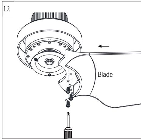
Install the blade by using the set screws provided. Align the 3 holes on in the blade with the screw holes in the motor and install the screws securely. Tighten screws securely. Repeat this process for remaining blades.
