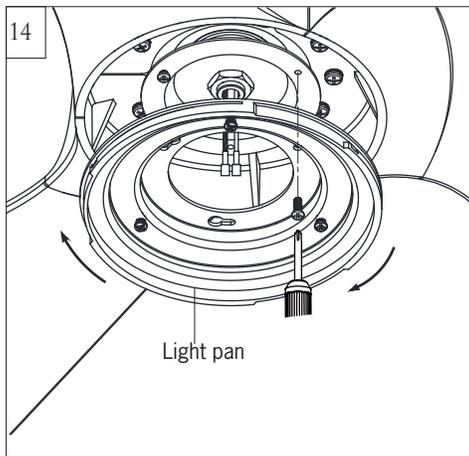
Attach the light pan onto the plate on motor, Place light pan over the lead wires from fan, aligning the keyhole slots on the light plate with the preassembled screws on the plate. Twist clockwise till lock. Reinstall the other screw. Tighten all screws securely.
