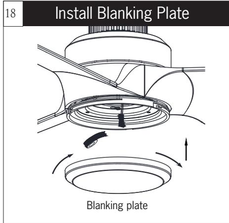
Isolate the quick connects with electrical tape.
