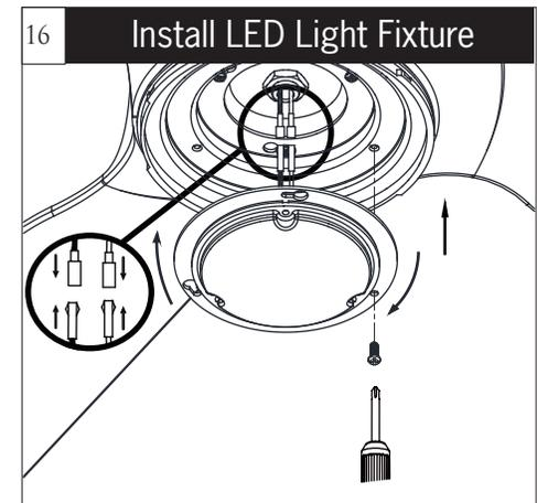
Connect white wire from fan to white wire from LED light fixture and then connect blue (or black) wire from fan to black (or blue) wire from LED light fixture. Be sure plugs connection clasped together firmly. Attach LED light fixture onto the light pan, aligning the keyhole slots on the LED light fixture with the preassembled screws on the light pan. Twist clockwise till lock. Reinstall the screw which was just removed. Tighten all screws securely.
