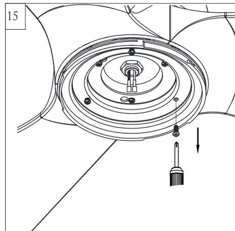
Loosen 2 and remove 1 preassembled screws from light pan. Keep screw.
