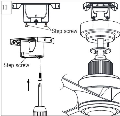
Partially loosen one and remove one preassembled step screw from mounting bracket (Do not remove the other set screws). Save the screw. Lift canopy up, aligning its keyhole slot with the preassembled step screw on mounting bracket and twist clockwise to lock in place. Reinstall the other step screw and tighten the screws securely. Attach canopy bottom cap onto canopy by aligning its holes with the step screws on mounting bracket and fix it with the magnet embraced in the cap.
