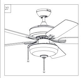
Thread pull chains through pull chain guides, and Install pull chains to preassembled pull chains on fan. Pull chains provided.
