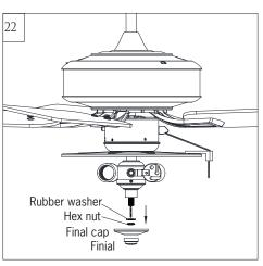
Remove finial, final cap, hex nut and rubber washer from light fixture. Keep the parts.
