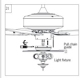
Remove the set screws from switch housing cap on top of light fixture. Keep screws.
