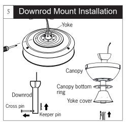
Partially loosen downrod set screws from yoke at top of motor assembly. Remove preassembled cross pin and keeper pin from downrod.
