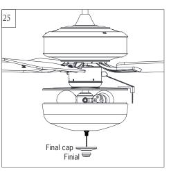
Align hole in center of final cap with thread rod, allowing pull chains to come through appropriate holes in the final cap, and push up. Thread center pull chain through hole in finial and secure glass to light fixture by tightening the finial. DO NOT OVER TIGHTEN the finial as glass may crack or break.
