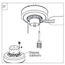
Remove shipping stabilizers from motor assembly.
