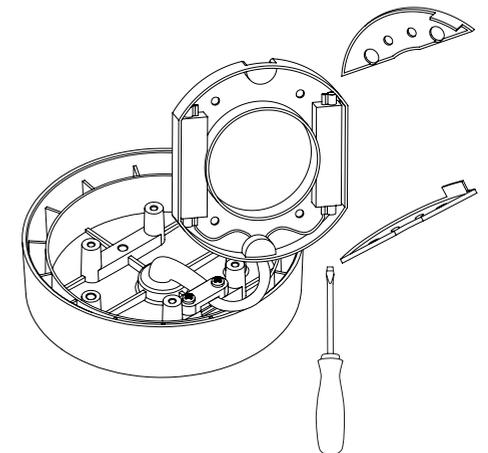
Pull up the bracket and use tool to take the lids off.
