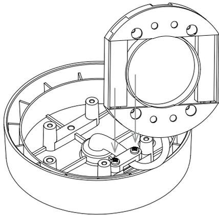
Put the lids back to the bracket and screw the wire release.
