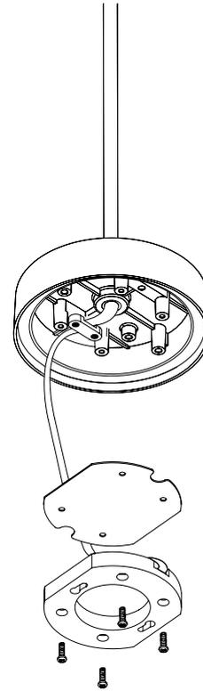
Assembly back after replacing the new cord.
