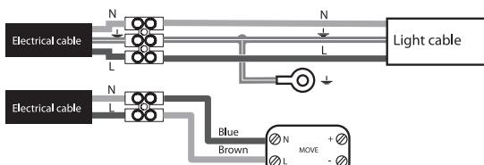
**EN** Drill the holes in the ceiling and position the screw anchors (D). Pass the electrical cable through the light fitting (C) and fix it to the ceiling with the screws (E). Connect the electrics according to the diagram and fix the electrical cable with the cable fastner (F).
