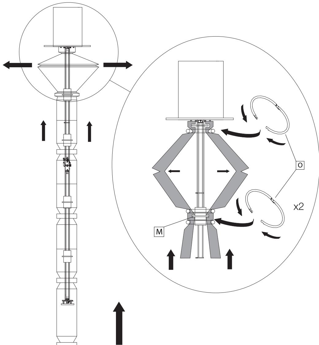
**EN** To place the middle clamps, stretch out the shade to raise it and be able to align the double exterior notches with the plastic part (M). Ensure that the interior groove of the shade fits over the plastic part (M). Place two clamps (O) in the two exterior waist of the shade (one above and one below).
