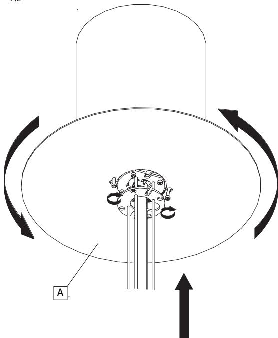
**EN** 7.1 Position the ceiling rose (B) on top of the fitting.
