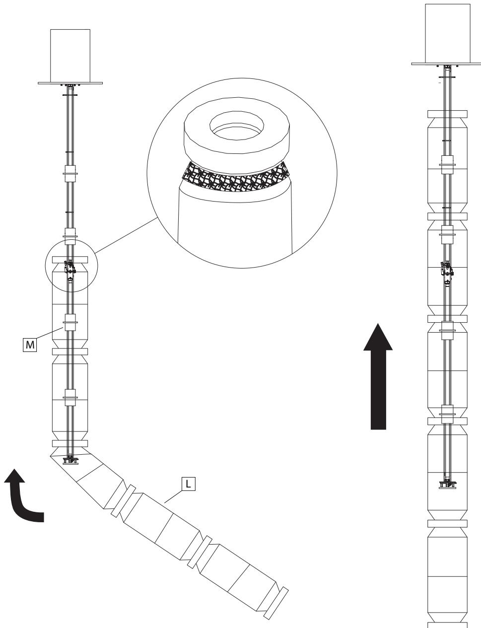
**EN** Place shade (L) carefully on to the light structure. Note that there is a specific way to place the shade. Ensure that the end with the black tape goes over first. Once the correct end has been identified, remove the tape. When placing the shade, it is necessary to stretch the fabric to fit over the components (M), do it without fear.
