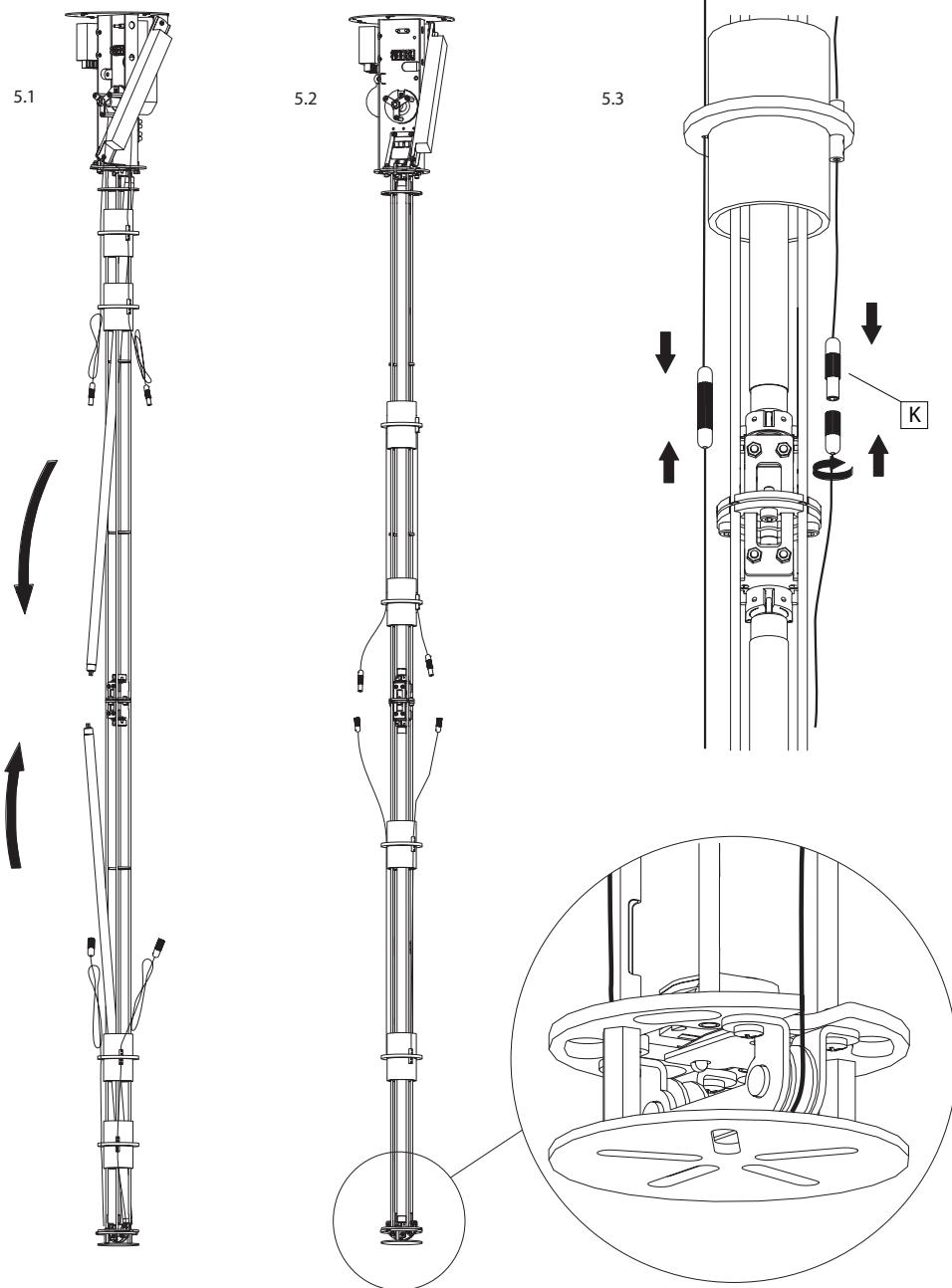
**EN** 5.1 Position and fix the fluorescent bulbs into the light structure.
