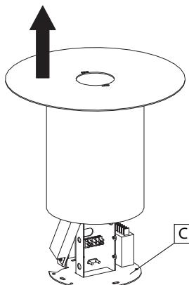
**EN** Loosen the screws (A) turning them a couple of times only without removing them. Turn the ceiling rose (B) slightly and separate it from the light fitting (C).
