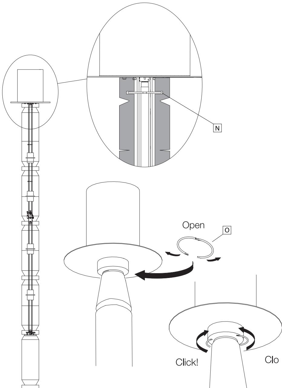
**EN** Align the top end of the shade with the plate (N) by continuing to slide the shade carefully on top of the structure, allowing the shade to hang down. Position and make sure that the top end of the shade is aligned with the plate. Open and place the first clamp (O) around the top waist of the shade and close the clamp to fix the shade.
