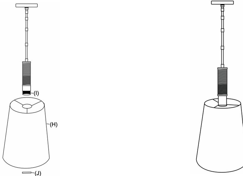
7. Insert one (1) **60 watt max E26 medium base bulb** (not included) or one (1) **9-watt max LED light bulb** (not included). To avoid the risk of fire, do not exceed the recommended lamp wattage.
