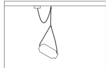
8. Slide the Canopy up to the ceiling and secure in place by tightening the Knurled Nut over the Threaded Rod.
