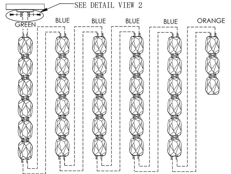
Each string of lights is identified by colored straps. Remove straps before installing. Connect sections as shown in the figure above. First, connect Green section to canopy, then attach Blue middle sections. At the end, attach Orange end section.
