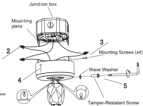
NOTE: Align connection so that tabs marked with A contact each other.
