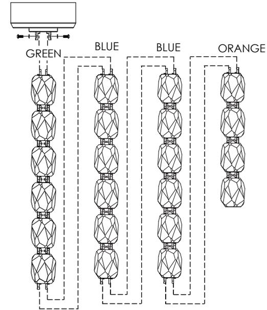
Each string of lights is identified by colored straps. Remove straps before installing. Connect sections as shown in the figure above. First, connect Green section to canopy, then attach Blue middle sections. At the end, attach Orange end section.
