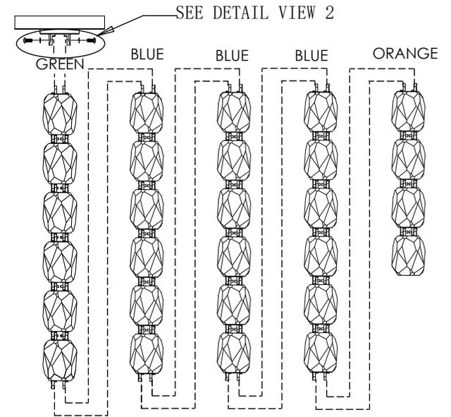
Each string of lights is identified by colored straps. Remove straps before installing. Connect sections as shown in the figure above. First, connect Green section to canopy, then attach Blue middle sections. At the end, attach Orange end section.
