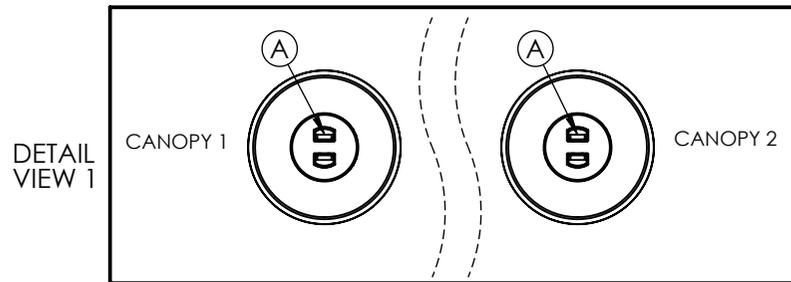
REPEAT STEPS 1-4 FOR BOTH CANOPIES. ORIENTATION MUST BE AS SHOWN IN DETAIL VIEW 1. TABS MARKED WITH A MUST BE IN LINE ON BOTH CANOPIES
