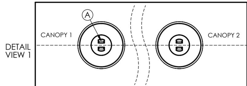
REPEAT STEPS 1-4 FOR BOTH CANOPIES. ORIENTATION MUST BE AS SHOWN IN DETAIL VIEW 1. THE TWO CANOPIES MUST BE MOUNTED IN LINE AS SHOWN.
