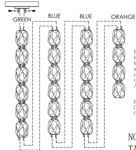
Each string of lights is identified by colored straps. Remove straps before installing. Connect sections as shown in the figure above. First, connect Green section to canopy, then attach Blue middle sections. At the end, attach Orange end section.
