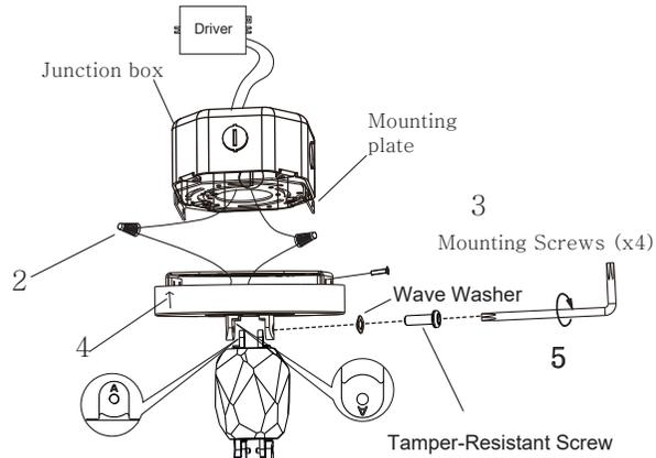
NOTE: Align connection so that tabs marked with A contact each other.
