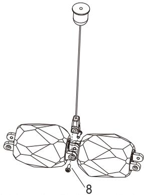
**Special Attention:** During installation, 12mm hex socket post screws should be used to avoid danger
