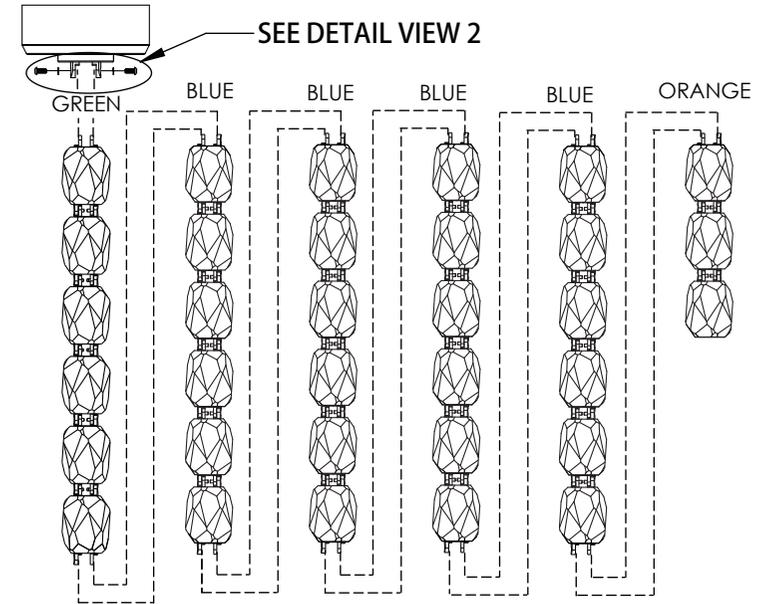
Each string of lights is identified by colored straps. Remove straps before installing. Connect sections as shown in the figure above. First, connect Green section to canopy, then attach Blue middle sections. At the end, attach Orange end section.
