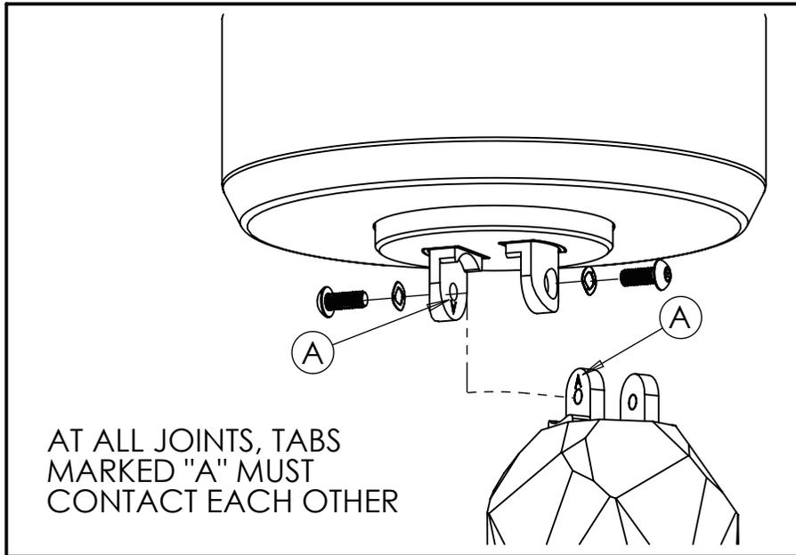
AT ALL JOINTS, TABS MARKED "A" MUST CONTACT EACH OTHER
