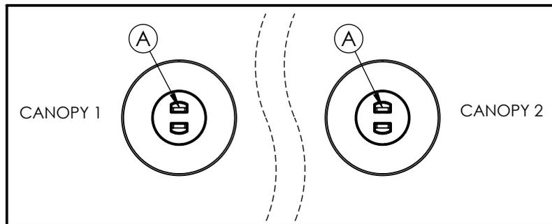
REPEAT STEPS 1-4 FOR BOTH CANOPIES. ORIENTATION MUST BE AS SHOWN IN DETAIL VIEW 1. TABS MARKED WITH A MUST BE IN LINE ON BOTH CANOPIES
