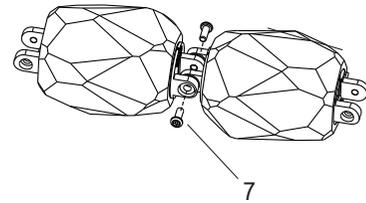
REMOVE SCREWS FROM CENTER CONNECTION OF YELLOW TAGGED SECTION OF LIGHTS
