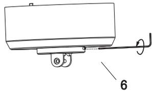
Use an Allen wrench to unscrew the set screw for 3-4 turns, about 2-3mm
