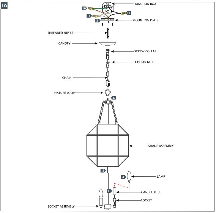
If necessary, screw the short end of the threaded nipple tightly onto the mounting plate, then screw the screw collar onto the threaded nipple.
