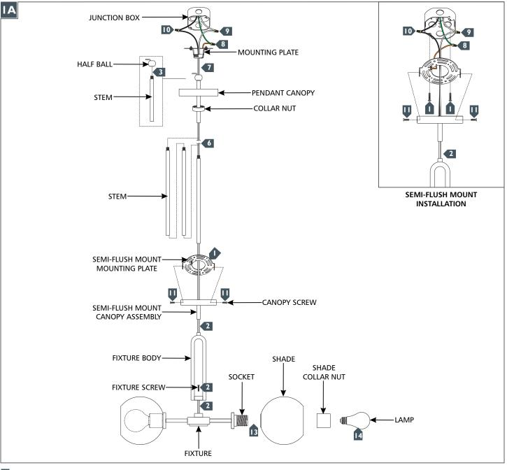
**For Semi-Flush Mount Installation Only**: Secure the semi-flush mount mounting plate to the junction box.
