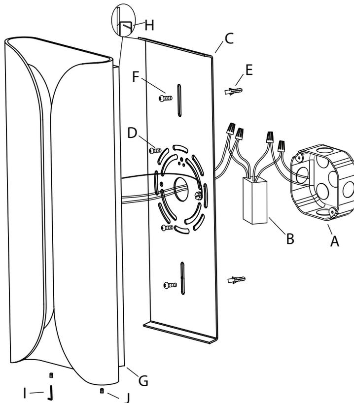
1. Shut off power to the outlet box (A).
