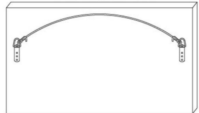
**The weight of the mirror not properly distributed places a strain at one point on both wire and hangers.**
