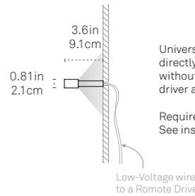
Universal bracket mounts directly to a wall with or without back plate in remote driver applications only.
