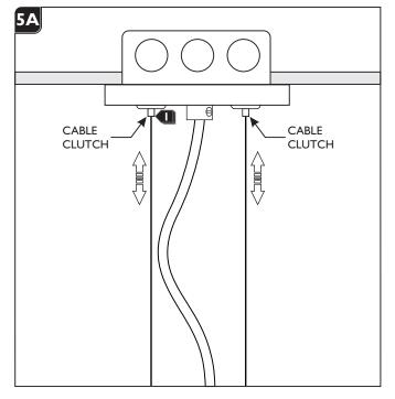
Adjust the aircraft cables until the fixture is level; feed the cable into the cable clutch to raise the fixture and push in on the cable clutch nipple to release the cable and lower the fixture.
