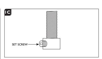
Doosen (Do Not Remove) the set screw on the strain relief.
