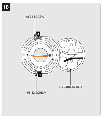
Install the mounting plate onto the electrical box with the two #8-32 screws provided.
