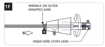
8 Keep pushing the coaxial cable into the connector while rotating the connector to ease feeding the inner wire into the tip of the connector. The outer wrapped wire will start wrinkling while being inserted another 1/2" into the connector.
