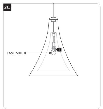
4 Push the lamp shield onto the spring clip.
