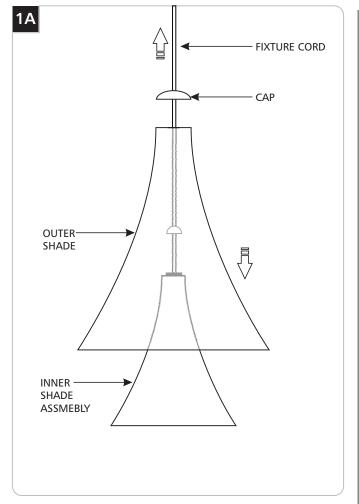
1 Feed the fixture cord through the outer shade and cap, then gently rest the outer shade on the inner shade assembly.
