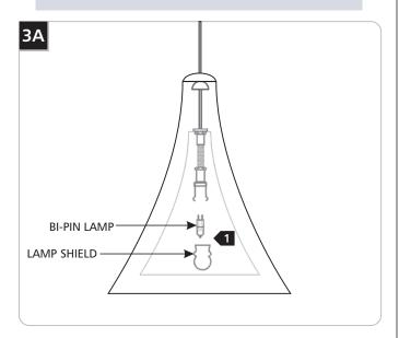
1 Remove the lamp shield and the old lamp.
