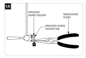
1 If applicable accessory fits tight or loose onto the Aero fixture, then carefully bend the grooved shade holder tabs in or out slightly with needlenose pliers.
