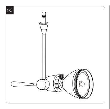
Line up the lamp pins with the socket holes. Insert the MR16 lamp pins into the socket holes, simultaneously push the accessory shade onto the grooved shade holder.
