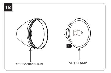
Use MAX 50 Watt, MR16 Front Cover Halogen Lamp.
