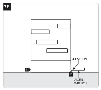
Carefully place the power line/cord inside the fixture, install the fixture onto the base plate, and secure it in place by tightening down the set screws.
