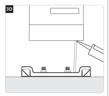
Caulk around the power line/cord where it enters the cord grip with waterproof construction sealant.
