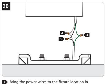
Bring the power wires to the fixture location in accordance with local electrical codes.
