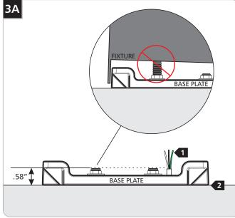
**Warning:** the mounting plate placement is off-center in relation to the center of the fixture on some models. Make sure to place the fixture in the desired location and determine the correct mounting plate placement before installing the mounting plate.
