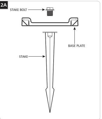
Attach the stake to the base plate by tightly screwing down the provided stake bolt through the center hole of the base plate and the stake.
