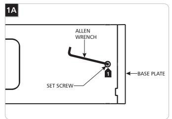
Loosen (Do Not Remove) the four set screws on column base with the provided Allen wrench and remove the base plate.
