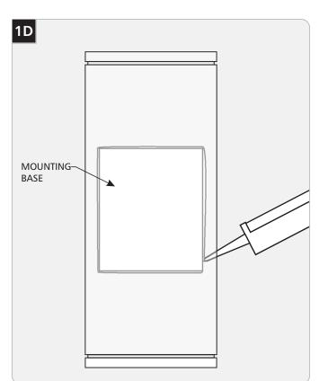
**For wet locations**, caulk around the mounting base with waterproof construction sealant.
