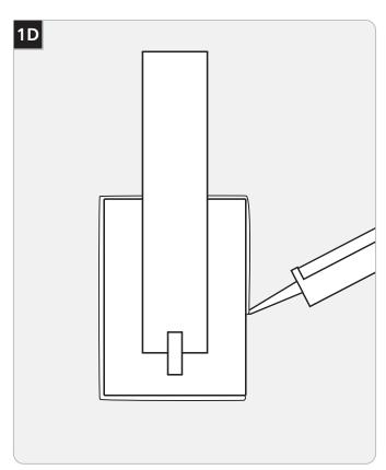
**10** For wet locations, caulk around the base with waterproof construction sealant.
