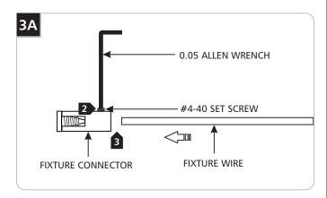
**NOTE:** Use this installation for both bare and insulated Kable Lite cables.
