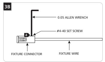
Tighten the #4-40 setscrew with the 0.05 Allen wrench.
