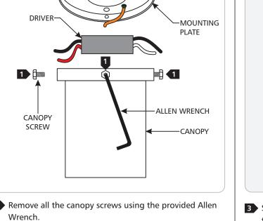
2 Remove the mounting plate and driver from the canopy.
