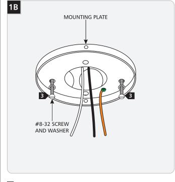
3 Secure the mounting plate to the electrical box with the two washers and #8-32 screws provided.
