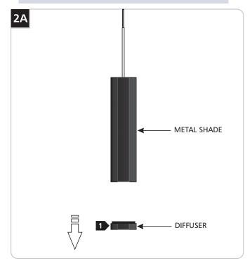
1 Remove the diffuser by supporting the metal shade and pulling down on the diffuser to separate it from the metal shade.
