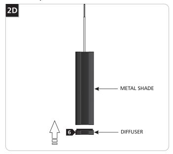
6 Install the diffuser by pushing it firmly into the bottom of the metal shade.
