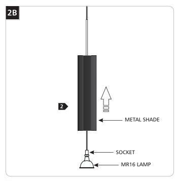
Move the fixture's metal shade up to expose the socket.
