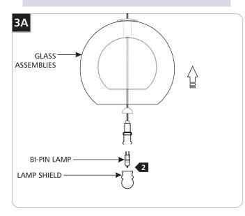
1 Lift inner and outer glass assemblies to expose socket
