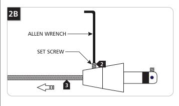
**2** Back out (do not remove) the set screw on the conical connector with the provided Allen wrench.
