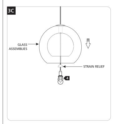
**5** Gently lower the inner and outter glass assemblies on to the strain relief.
