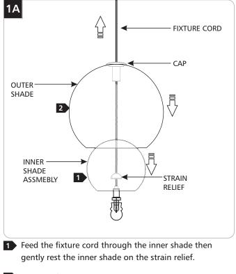
2 Feed the fixture cord through the outer shade and cap, then gently rest the outer shade on the inner shade assembly.
