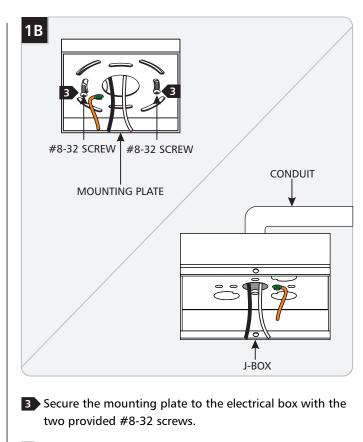
4 (Optional): If using the Exo J-Box connect the conduit or romex to any of the available knockouts.
