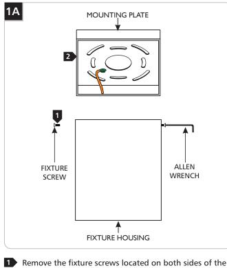
Remove the fixture screws located on both sides of the fixture housing using the provided Allen wrench.
