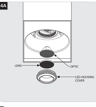
1 Unscrew and remove the LED housing cover.
