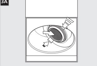
**WARNING:** Always squeeze the two tabs when adjusting the LED housing. Failure to do so will damage the finish.
