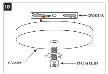
Remove the crossbar from the canopy by completely unscrewing the strain relief.
