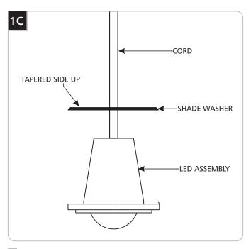
Feed the pendant cord through the shade washer and rest it on the LED assembly <u>tapered side up</u>.
