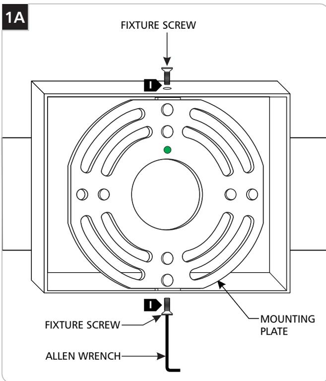
**1** Remove the fixture screws located on the top and bottom of the fixture base with the provided Allen wrench.
