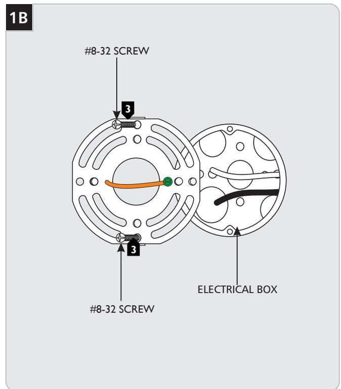
**3** Install the mounting plate onto the electrical box with the two #8-32 screws provided.
