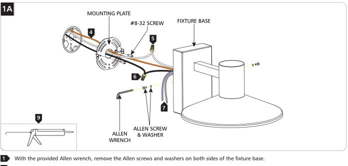
2 Remove the mounting plate from the back of the fixture.
