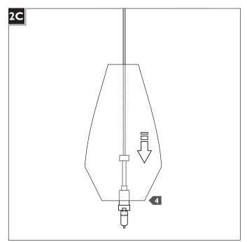
4 Lower the glass shade onto the socket assembly.
