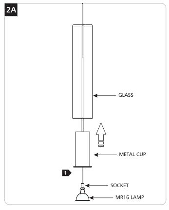
Move the fixture glass and metal cup up to expose the socket.
