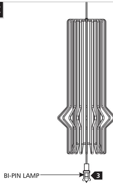
**3** Handle the new replacement lamp with a soft cloth to prevent the natural oils on the fingertips from collecting on the lamp. This will help extend the life of the lamp.
