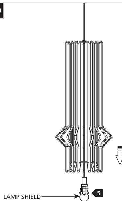
**5** Push the lamp shield onto the spring clip.
