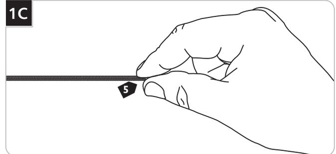
**4** Cut the coaxial cable to the desired length.
