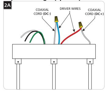
1 If shortening of the coaxial cords is necessary, take note of the wire connections and polarity from the coaxial cables to the driver and remove the wire nuts.
