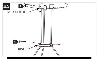
**CAUTION:** Make sure to support the fixture if fine leveling is necessary.
