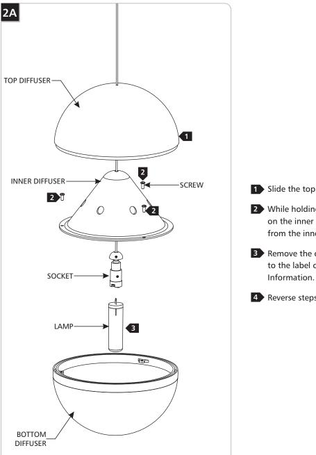
1 Slide the top diffuser up to expose the inner diffuser.
